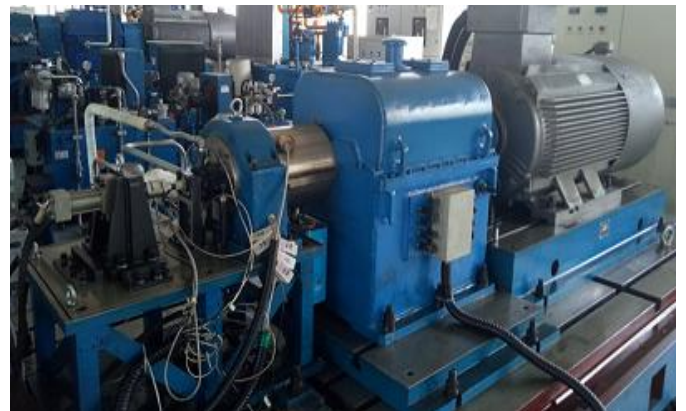
China's First High-Speed Rolling Bearing Test Rig with DN Values Exceeding 3 Million
