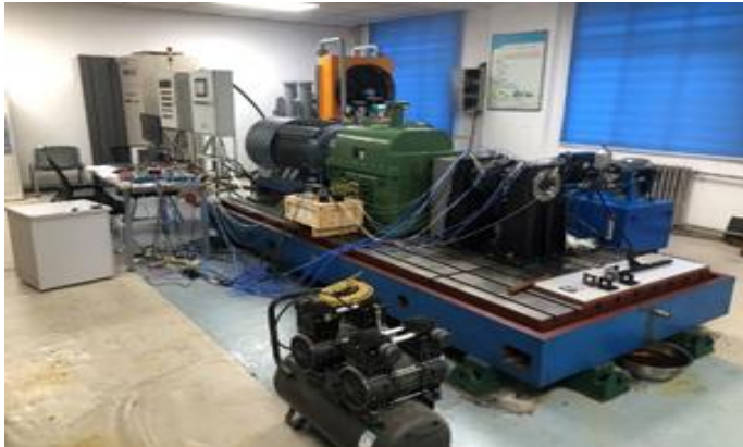
Comprehensive Test Platform for Performance Evaluation and Failure Validation of Sliding Bearings
